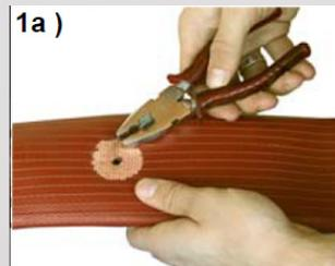
For this type of hose first of all remove the external cover around the damage back to the textile reinforcement.
