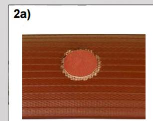
The size of the repair patch should be 2 mm smaller than the removed external cover.
